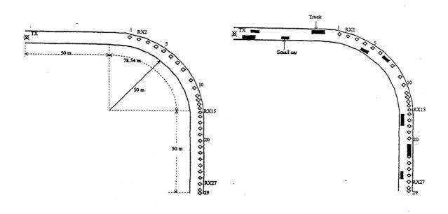
Fig. 3 Top view of the tunnel. TX denotes the transmitter.  $\blacklozenge$  denotes the receiver.
