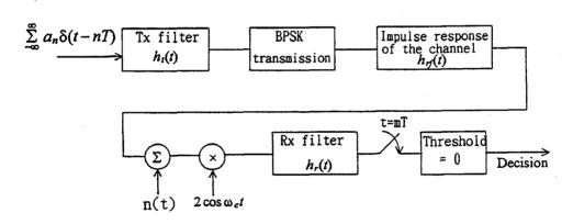
Fig. 2 Block diagram of the simulated communication system.
