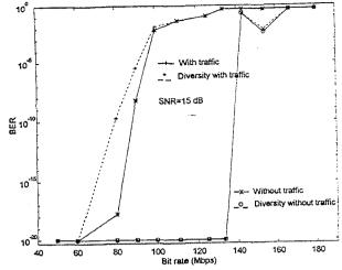
Fig. 8 Dependence of BER on transmission rate for the cases of tunnels with and without traffic. SNR is 15 dB. The receiver is located at RX27.
